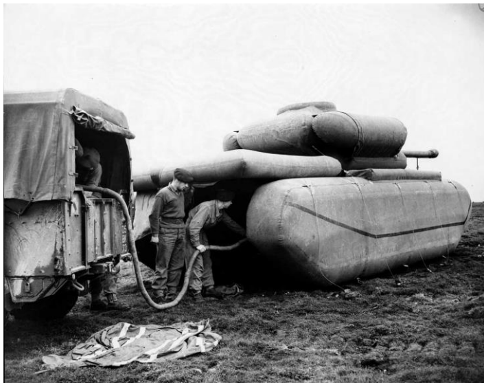
Ghost Tank being filled with air
